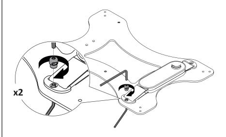
4 Hand strap installed on hardware mount\*
